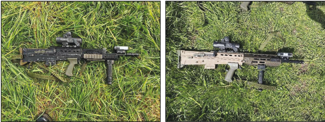
Figure 4 - Comparison of SA80 L85 A2 (left) and A3 (right)
