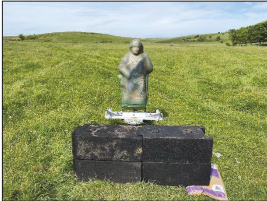
Target system mounted on lifting mechanism and Location of Miss and Hit (LOMAH) bar
